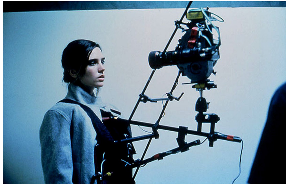
Fig. 1: The so-called 'Snorricam' used to shoot Requiem for a Dream (Darren Aronofsky, 2000). Courtesy John Baer (© John Baer 1999)
